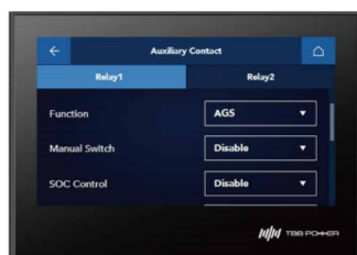
Generator AGS Control Setting
