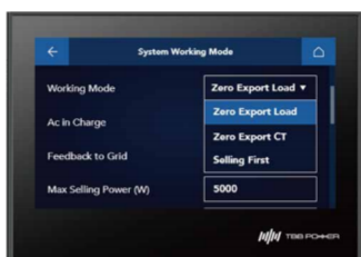
Working Mode Setting: Zero export to load, Zero export to CT and Selling first
