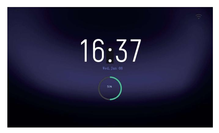
Touch any part of the screen to navigate to the homepage. On this page, all power data and the battery's state of charge can be monitored. WiFi connection settings can be configured in the Settings menu.
