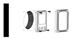
**Step 1:** Mark and cut an appropriately-sized hole in the surface for the cable and rear of the screen
