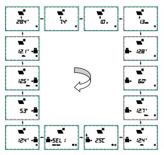
**Display Loop:** PV voltage → PV current → PV power → Battery power → BATT1 voltage → BATT1 current → Max. BATT1 voltage → Min.BATT1 voltage → BATT1 temperature → BATT1 battery type → BATT2 voltage → BATT2 current → Max. BATT1 voltage → Min.BATT2 voltage → PV voltage
