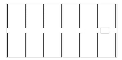
Break the adhesive lines in the middle of the solar panel with a gap of 70-100 mm. This will even the pressure and allow for additional escape routes for air and water if the edges of the solar panel are not sealed at the end of the installation.
