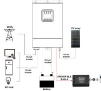
**Note:** The Bluetooth module only supports one-to-one communication (i.e., a Bluetooth module can only connect one controller, inverter, or inverter/charger). Detail connection cable refers to the connected device accessories list.
