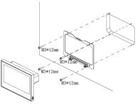
3) .Wall MountingInstallation Diagram( Use M4 screws)
